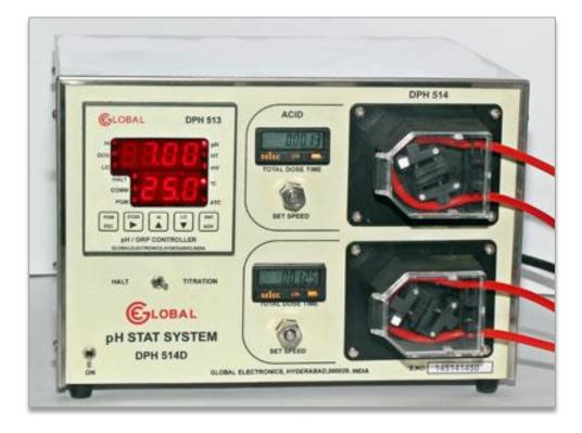
This is specially designed for critical pH control in Laboratory processes and experimentation.
